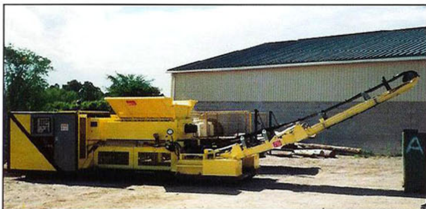
ST-100H Roll-Off Shredder on location processing empty propane cylinders.
